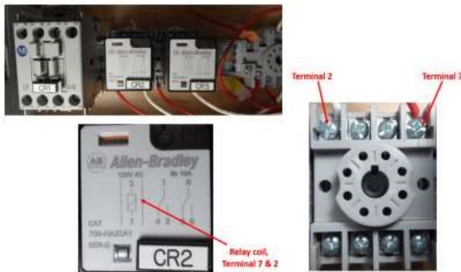
Figure 4: Connections for the ice cube relay coils used in this lab
